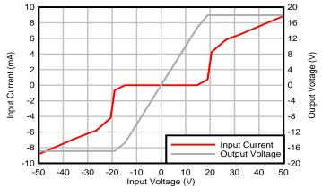
Figure 63. Input Current vs Input Overvoltage
