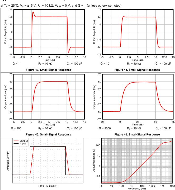
Figure 47. Large-Signal Step Response
