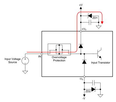
Figure 62. Input Current Path During an Overvoltage Condition
